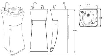
INLET: 860mm ABOVE BASE 100mm LEFT OF CENTRE LINE (from back) OUTLET: 860mm ABOVE BASE 30mm LEFT OF CENTRE LINE (from back)
